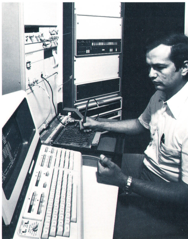
Fig. 1. Model DTS-70 Digital Test System gives fast and accurate go/no-go tests of complex digital circuit boards. If a board fails a test, the software presents messages to guide the operator in using the probe to find the fault.
